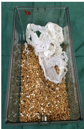
IVC – Individually Ventilated Cage Allentown 18cm(w) x 38cm(l) Total floor area 684cm 2
