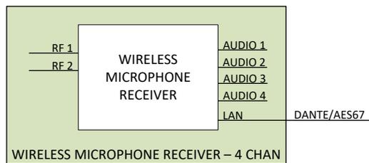
Image: Audio System IP – Wireless Microphone Receiver
